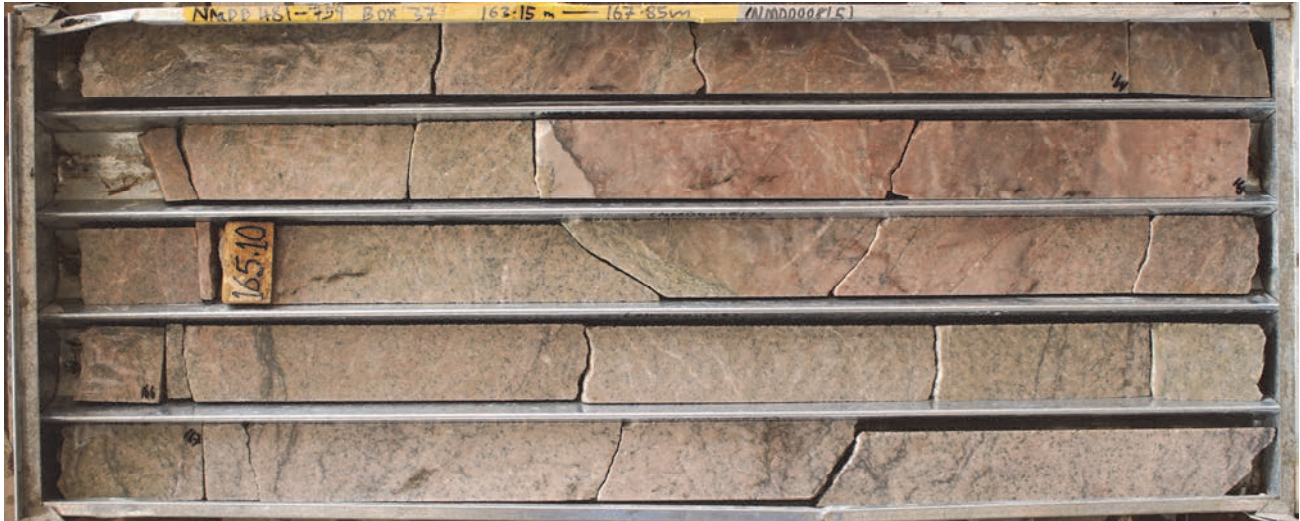
Figure 9: Hydrothermally altered monzonite granitoids containing pyrite blebs and arsenopyrite sulphides (NMDD481-759)
