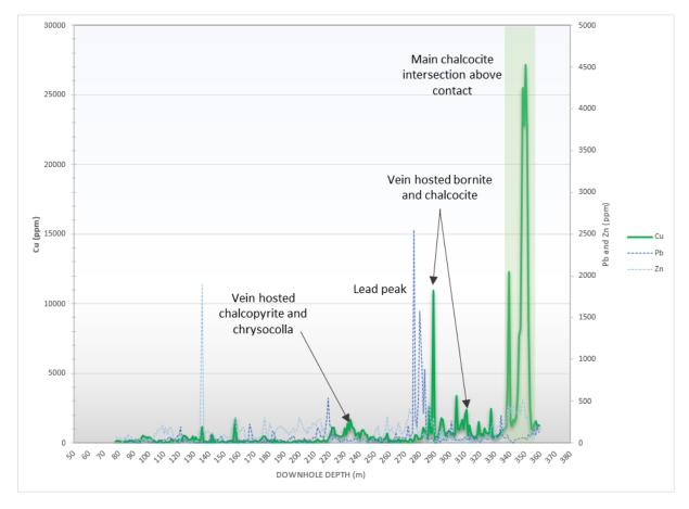
Figure 2. Graphical illustration of pXRF composite 1m sample measurements for the complete NCP11-B hole. Results confirm the abundance of visual copper mineralisation in drill logs. Distinct mineral zonation from chalcocite-bornite-chalcopyrite from the Ngwako Pan Formation contact is apparent.
