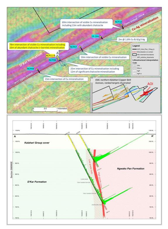
Figure 3. Plan view (above) illustrating drill positions on airborne magnetic data. Section (below) through NCP11-B and NCP08 illustrating mineralisation (green plot) related to the D'Kar / Ngwako Pan formation contact. Note the gentle folding of the contact interpreted from structural measurements of oriented core.
