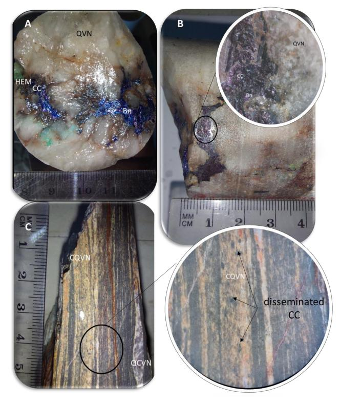
Figure 1. Examples of mineralisation intersected in NCP11-B. (A and B) Bornite (Bn) and chalcocite (CC) mineralisation hosted in a quartz vein, (C) Chalcocite mineralisation in carbonate (+- quartz) veins in the altered marl unit above the D'Kar – Ngwako Pan Formation contact.
