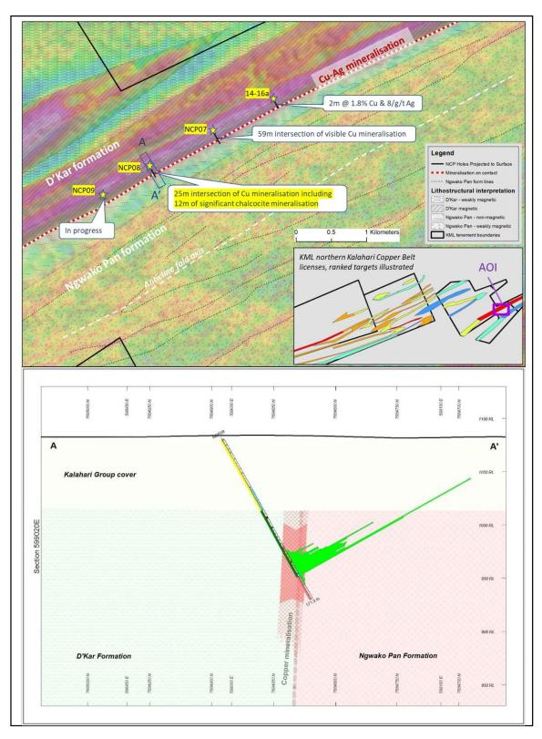
Figure 3. Plan view (above) illustrating drill positions on airborne magnetic data. Section (below) through NCP08 illustrating mineralisation (green plot) related to the D'Kar / Ngwako Pan formation contact.
