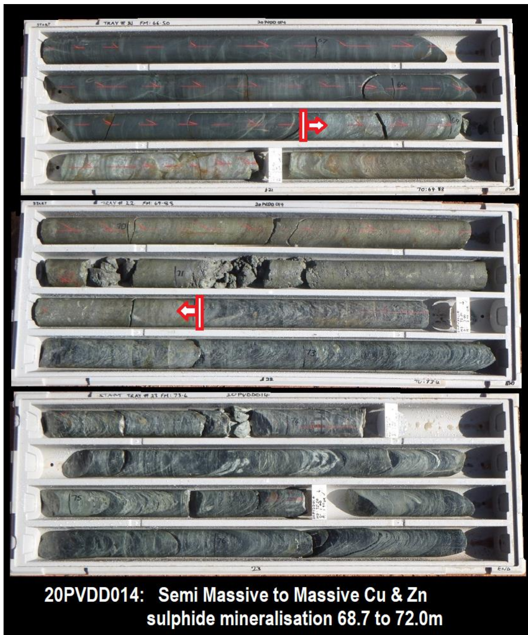
Figure 1: VHMS Mineralisation in Schwabe Prospect DC hole 20PVDD014
