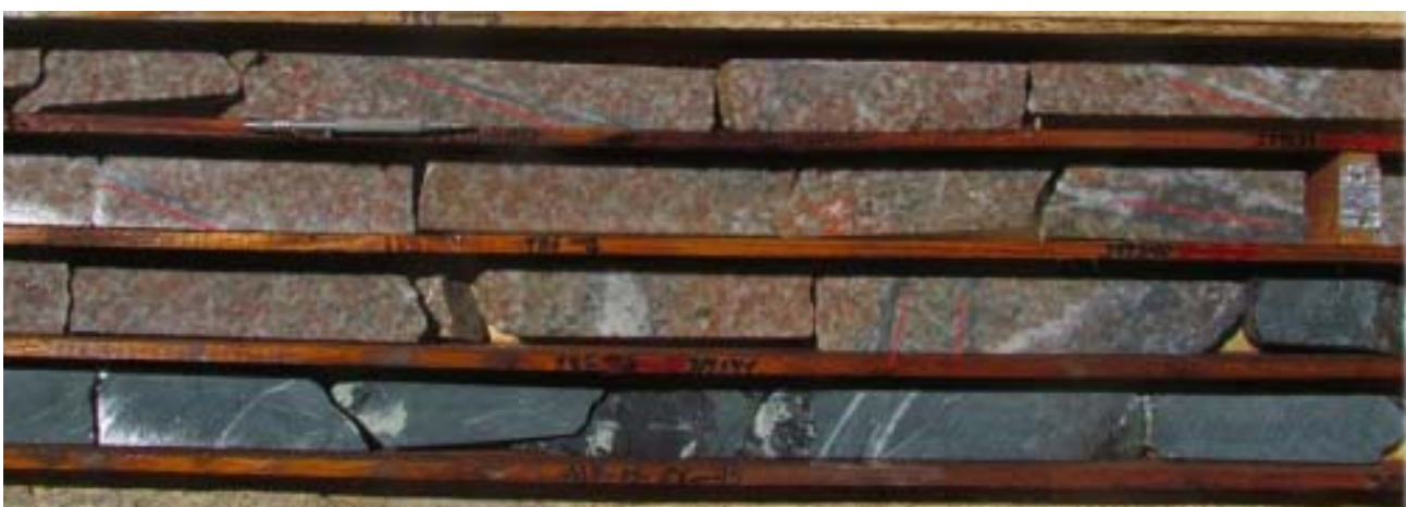
Figure 5: High-grade mineralised section of MD-01 showing veinlets (marked in red) at both a low angle and high angle to the core axis
