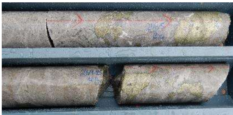
High grade copper in hydrothermal infill breccia CAE hole # 14,: 269m depth. Interval 268m-270m: 2m @ 4.21% Cu ,0.39 g/t Au, 60.5 g/t Ag.
