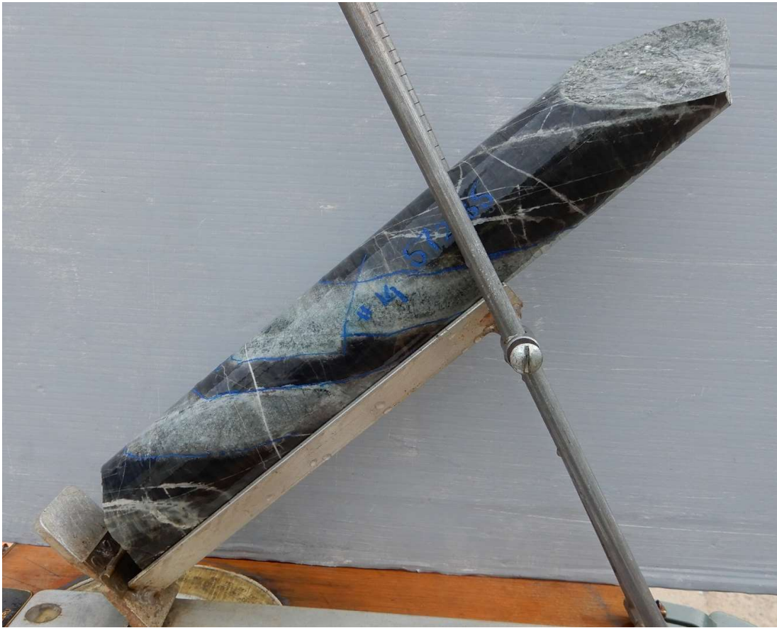
Fig 20. HQ Full Core oriented in Core Orienting Frame, hole drilling to east (hole bearing 090 degrees mag) inclined at 43 degrees, view looking south . Hole 22CAEDD014 at 572.85m :Fine grained siltstone thinly interbedded with lighter coloured silica sericite altered sandstone. Beds dipping 18 degrees to east ( 085 magnetic.)
