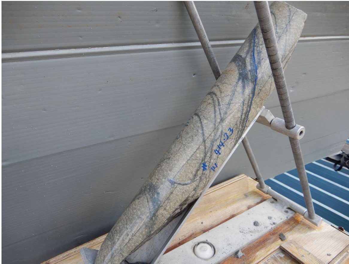
Fig 18. HQ Full Core oriented in Core Orienting Frame, hole drilling to east (hole bearing 088 degrees mag) inclined at 49 degrees, view looking south west. Hole 22CAEDD014 at 414.5m :Sericite altered diorite porphyry cut by sheeted veins of pyrite with quartz alteration selvages. Trend of veins are dipping 74 degrees to east south east ( 115 mag). Similar styles of veining and phyllic alteration are characteristic of many porphyry style deposits.
