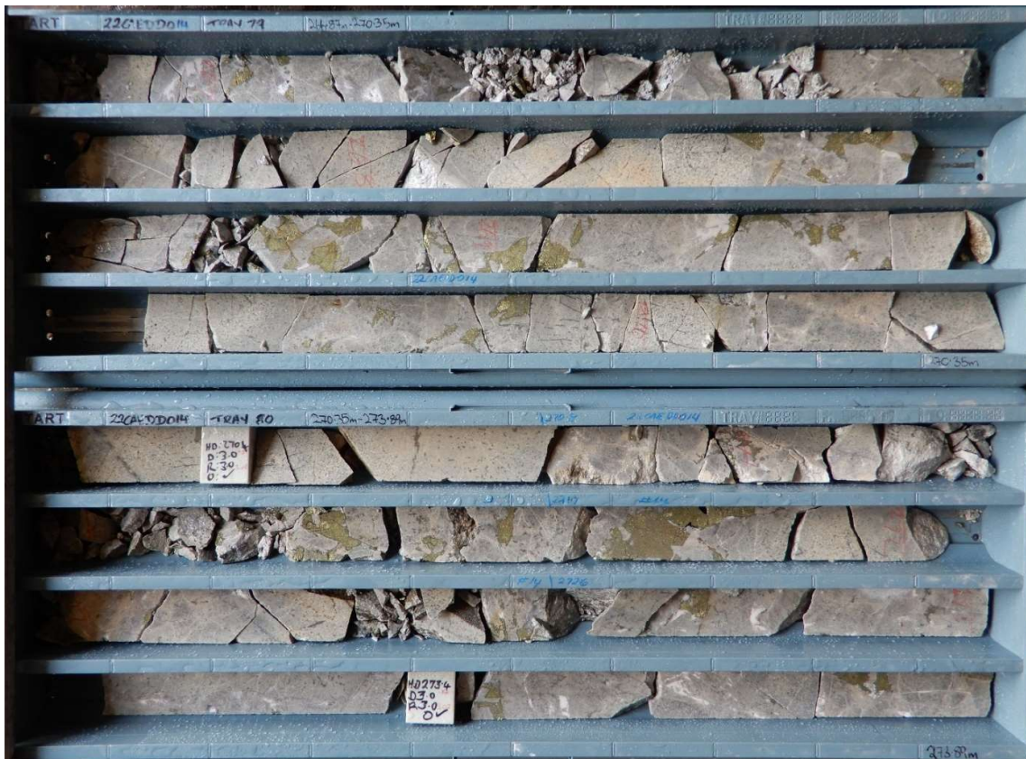
Fig 15. HQ Half Core photo hole 22CAEDD0014, around 270m , Chalcopyrite – pyrite-quartz – calcite infill between angular clasts of sericite altered diorite. Interval 267m-272m : 5m grading 3.26% Cu, 0.4 g/t Au, 47.2 g/t Ag, 4.89% S.
