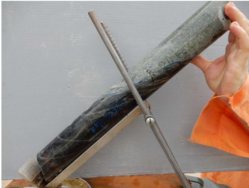
Fig 21. HQ Full Core oriented in Core Orienting Frame, hole drilling to east (hole bearing 090 degrees mag) inclined at 43 degrees, view looking south. Hole 22CAEDD014 at 569.85m: Fine grained dark hornfelsed siltstone interbedded with lighter coloured silica sericite altered feldspathic sandstone. Beds dipping 28 degrees to east (080 magnetic.), running down core.
