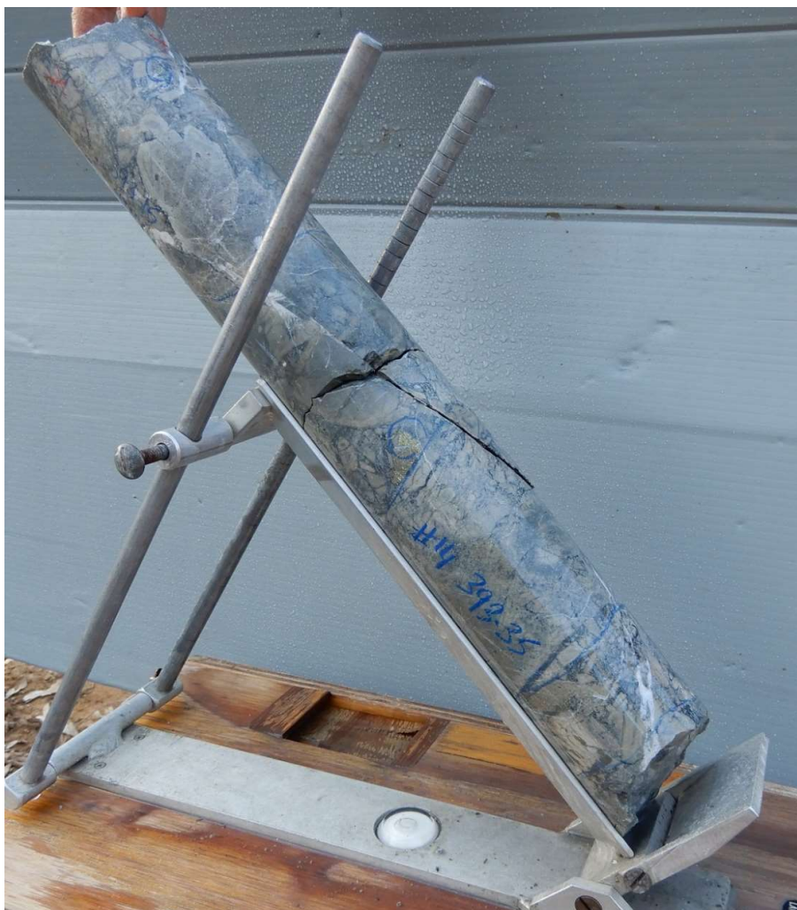
Fig 17. HQ Full Core oriented in Core Orienting Frame, hole drilling to east (hole bearing 088 degrees mag) inclined at 49 degrees, view looking north. Hole 22CAEDD0014 at 393.35m :Polymict clast supported breccia with angular to subangular clasts of hornfels, some porphyry and diorite. Chlorite , pyrite, calcite some rare chalcopryite infill, minor rock flour matrix. General alignment of flat clasts in breccia is dipping 45 degrees to west.
