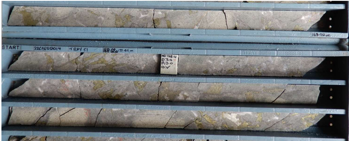
Fig 14. HQ Half Core photo hole 22CAEDD0014, around 168m , Chalcopyrite – pyrite-quartz – calcite infill between angular clasts of sericite ankerite altered diorite. Interval 167m-171m : 4m grading 3.48% Cu, 0.47 g/t Au, 49.9 g/t Ag, 7.68% S.
