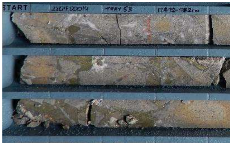
Hydrothermal infill breccia altered diorite clasts, chalcopyrite -pyrite -calcite-quartz infill. CAE hole # 14: 174m-177m depth. 3m @ 1.58% Cu, 0.69 g/t Au, 24.3 g/t Ag,
