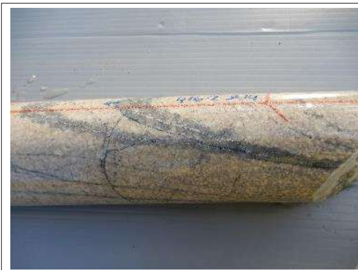
Fig 18. HQ Full Core oriented in Core Orienting Frame, hole drilling to east (hole bearing 088 degrees mag) inclined at 49 degrees, view looking south west. Hole 22CAEDD014 at 414.5m :Sericite altered diorite porphyry cut by sheeted veins of pyrite with quartz alteration selvages. Trend of veins are dipping 74 degrees to east south east ( 115 mag). Similar styles of veining and phyllic alteration are characteristic of many porphyry style deposits.
