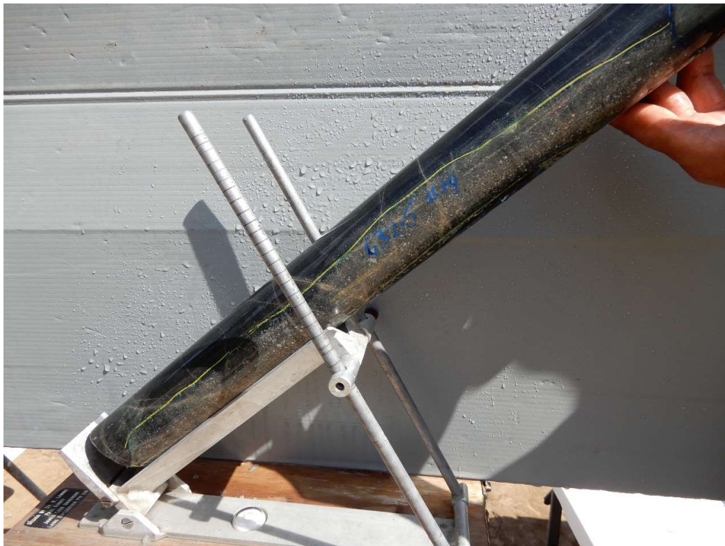
Fig 22. HQ Full Core oriented in Core Orienting Frame, hole drilling to east (hole bearing 091 degrees mag) inclined at 40 degrees, view looking south. Hole 22CAEDD014 at 632.5m: Fine grained hornfels siltstone thinly interbedded with coarser grained feldspathic sandstone, probably volcanic derived. Beds dipping 39 degrees to east (090 magnetic.), running down core ie. Hole drilling exactly down dip of stratigraphy.
