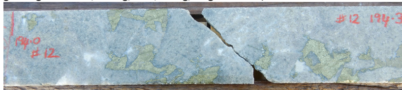
Chalcopyrite – pyrite-quartz – calcite infill between angular clasts of sericite altered diorite. CAE hole # 12, 194.3. Interval 194m-195m grading 4.52% Cu, 0.94 g/t Au, 57.3 g/t Ag, 8.04% S,
