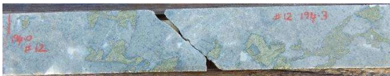
Fig 14. HQ Half Core photos hole 22CAEDD0012, 194.3, Chalcopyrite pyrite-calcite infill in monomict crackle brecciated diorite.. Interval 194m-195m assays 1m @ 4.52% Cu, 0.94 g/t Au, 57.3 g/t Ag, 8.04 % S
