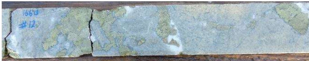
Fig 11. HQ Core photos hole 22CAEDD0012, 166.0m, Chalcopryite – pyrite-quartz – calcite infill between angular clasts of sericite altered diorite. Interval 166m-167m grading 3.05% Cu, 0.56 g/t Au, 55.2 g/t Ag, 9.62% S
