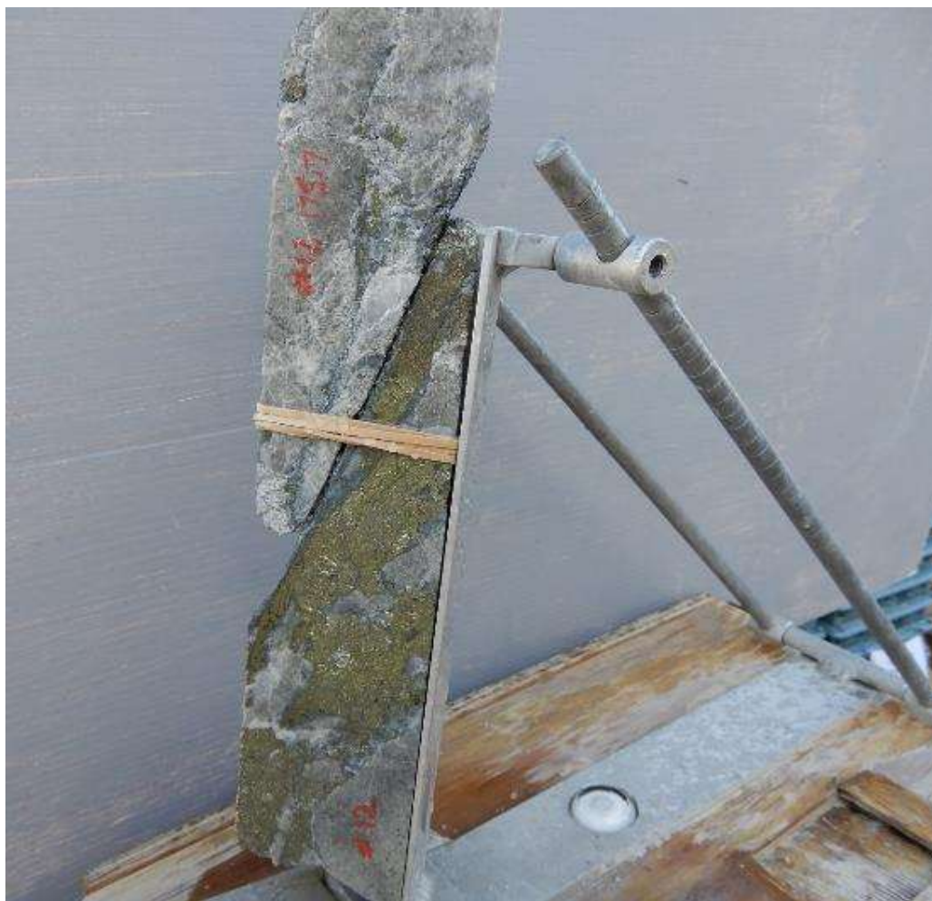
Fig 12. HQ half Core oriented in Core Orienting Frame, hole drilling north at 80 degrees, looking south-east. Contact of semi-massive chalcopryite -quartz-calcite infill in structure trending east south- east (strike 120-300 magnetic bearing, dipping 65 degrees to north-east) in contact with strongly silica sericite altered diorite breccia. Hole 22CAEDD0012, 175.7m, Interval 175m-176m grading 2.45% Cu, 0.54 g/t Au, 50.6 g/t Ag, 7.86% S
