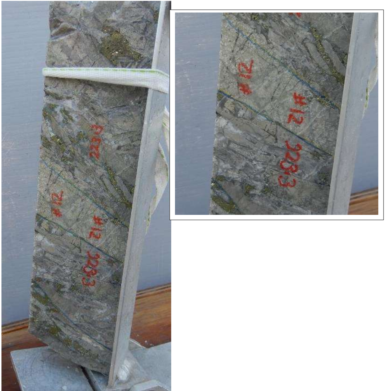
Fig 18. HQ half Core oriented in Core Orienting Frame, hole drilling north at 80 degrees, looking south-east. Splinter breccia dominated by tabular clasts of hornfels with pyrite-chalcopyrite, quartz calcite infill between clasts. Clasts are generally aligned and dip relatively gently to the south south-west. Overall attitude of the clasts is strike (110-290 magnetic bearing dip 45 degrees to south south-west). Hole is interpreted as drilling down long axis of the breccia, with clast alignment almost at right angles to drill direction. Hole 22CAEDD0012, 223.3m, Interval 223m-224: 1m grading 2.15% Cu, 3.17/t Au, 96.5 g/t Ag, 5.38% S.
