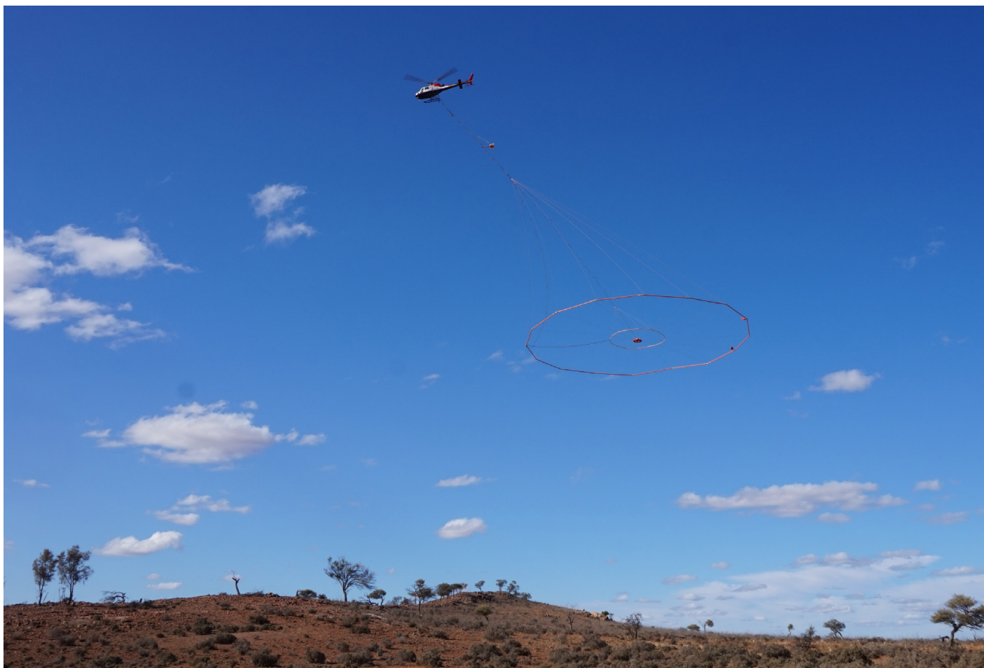
Figure 3. Airborne electromagnetic survey at the Thackaringa project 25km south-west of Broken Hill.
