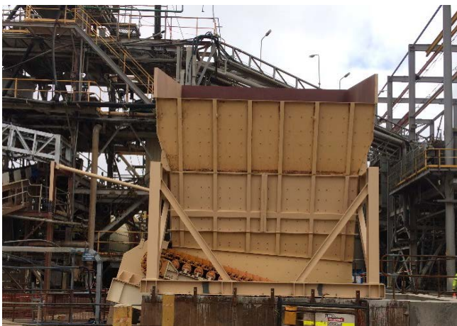
Photo 6: New Mill 1 feed hopper installed
