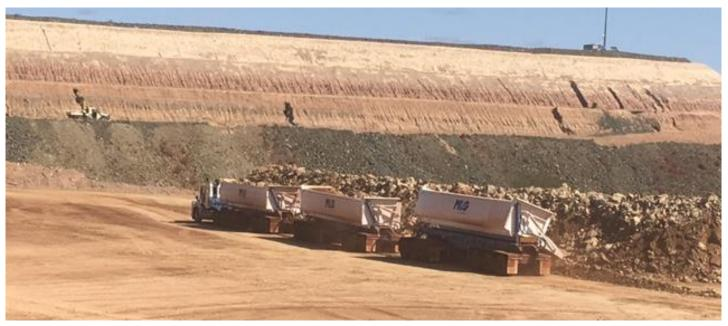
Photo 2: One of two MLG road trains hauling ore back to ROM
