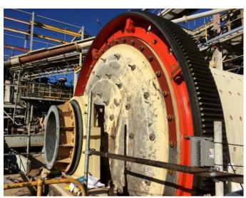
Photo 6: Mill 2 girth gear installed
