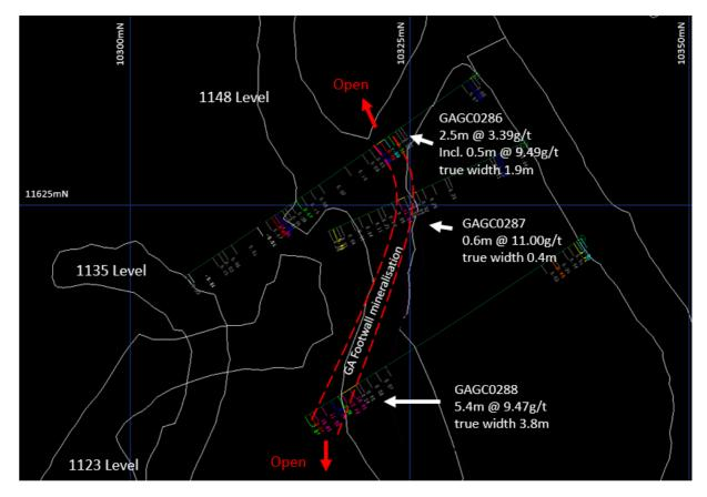
Figure 1: Plan view of footwall reef in situ below the stoped 1148 level.
