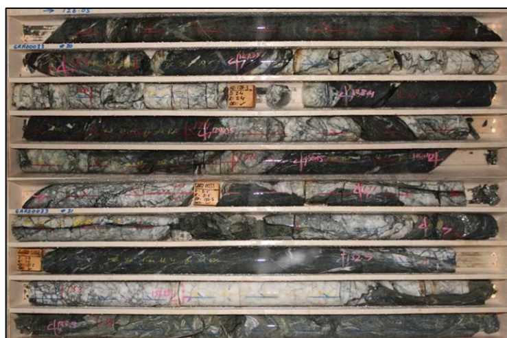
Photo 1: GARD0033, Golden Age Shear Zone and thick laminated quartz reef with assay results of 6.9m @15.5g/t
