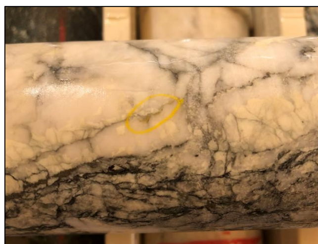
Photo 2: Visible Gold in GARD0034 (3.0m @ 2.11 g/t Au) to be re-assayed by screen fire assay
