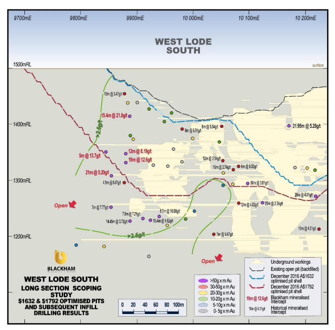
Figure 4. Long section through West Lode South showing extensions of mineralisation to the south of West pit. New mineralisation is likely to extend the planned PES pit further south.
