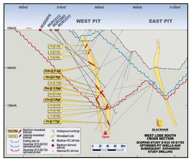
Figure 5. Section through West Lode South – drilling has confirmed broad high-grade mineralisation, likely to extend the planned PES pit deeper and further south.
