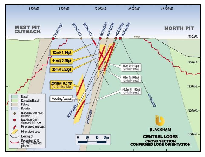
Figure 6. Cross section showing significant intercepts for the Central Lodes all of which are currently outside the reported resources (outside Dec'16 \$1792 shell).
