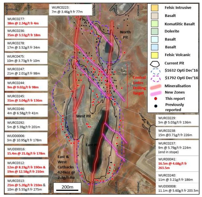
Figure 1. Plan view showing collar locations of latest drilling results (downhole widths quoted) and updated mineralisation interpretation in relation to pre-drilling pit optimisation shells. Note significant new mineralisation outside the current pit optimisations.
