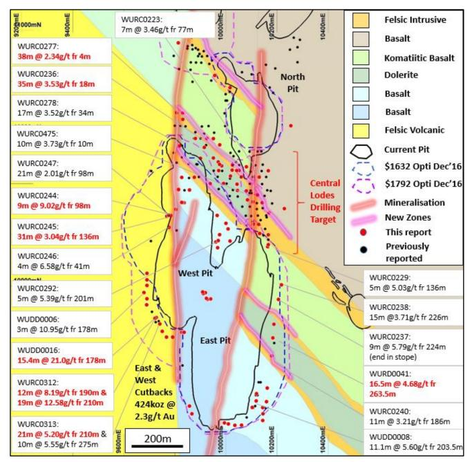
Figure 2. Plan view showing collar locations of latest drilling results (downhole widths quoted) and geological interpretation in relation to pre-drilling pit optimisation shells. Note significant new mineralisation outside the current pit optimisations.
