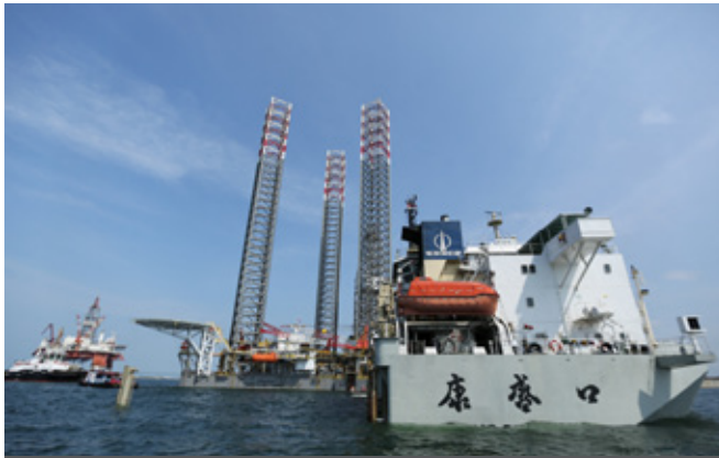
ENDEAVOUR BEING LOADED ONTO HEAVY LIFT VESSEL
