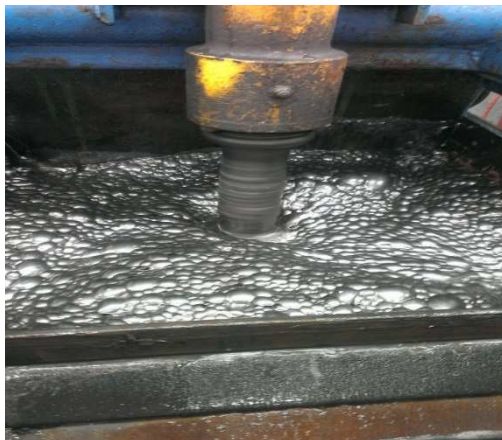
Free flowing well ordered froth conditions during bulk flotation resulting in less entrainment and excellent launder flow
