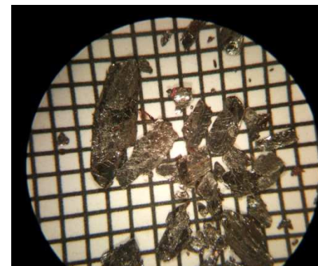
Extremely coarse graphite released by knapping Argent outcrop (The square scale grid is 1 mm)
