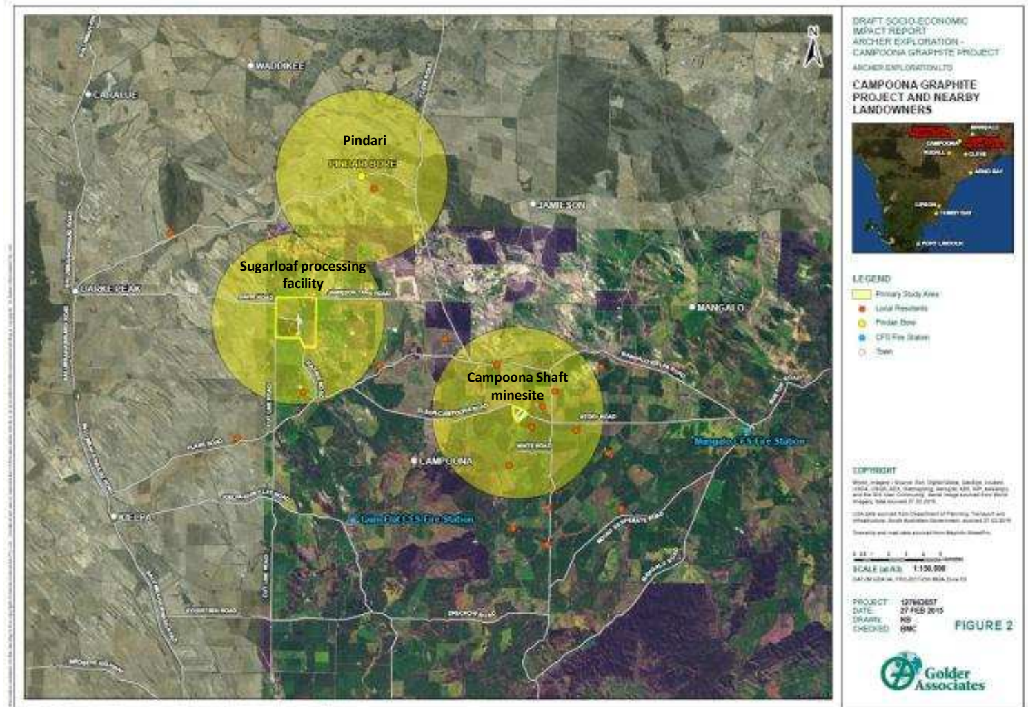
“Hub and spoke” development where satellite mines feed a centralised mineral processing facility
