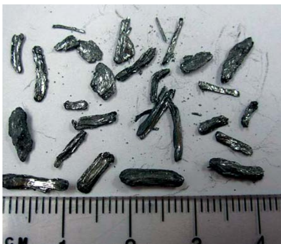
Flake aggregates from RC drill hole WG041 (98-99m)
