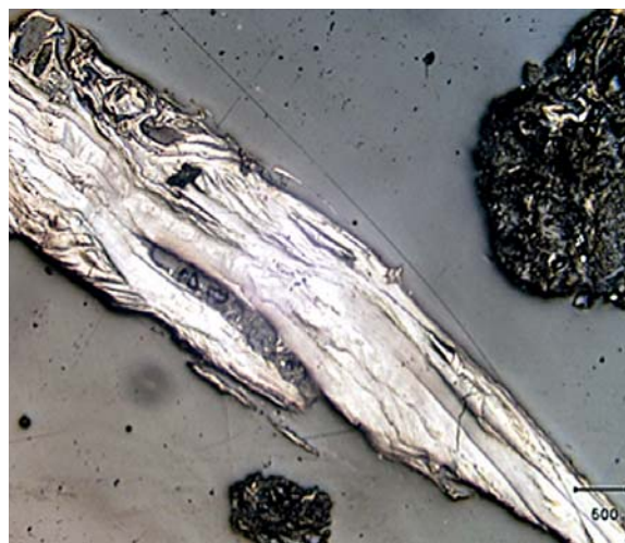
Sample 28727, Hole WG090, 74-75m. Large liberated flake, (x20), scale bar 500 \mu m.
