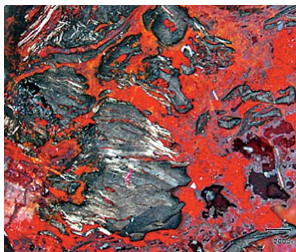
Sample 28718, Hole WG044, 73-74m. (PPL), (Xnic). Graphite scattered as individuals and composites, all enclosed within ochreous-red ferruginised ex-felspars and local micas.
