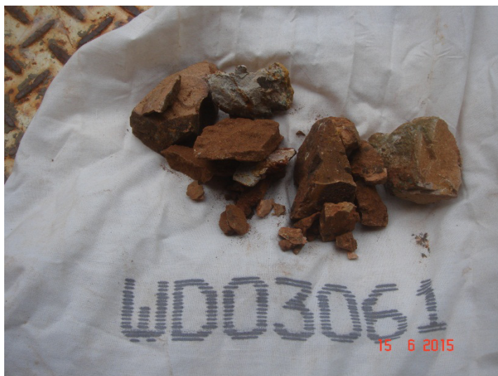
Plate 3. Example of material reporting 2.16%Cu
