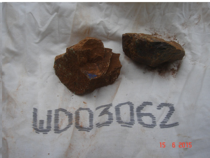
Plate 4. Example of material reporting 2.88% Cu
