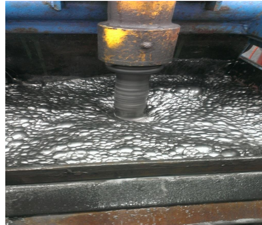
Free flowing well ordered froth conditions during bulk flotation
