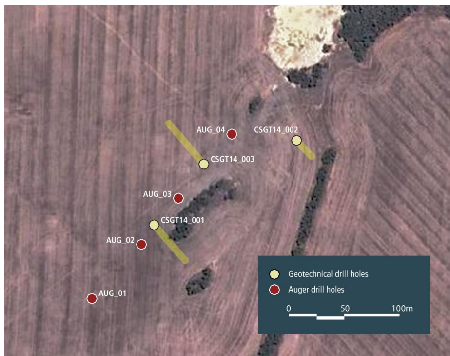
Plate 7. Location of Geotechnical (GT) and Auger (Aug) holes at Campoona Shaft
