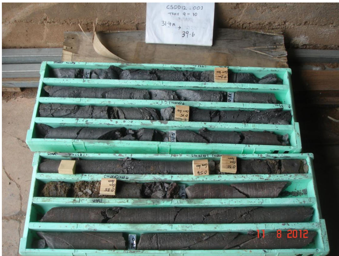
Plate 1. CSD12_001 core from 31.4 – 39.6m within zone of complete oxidation.
