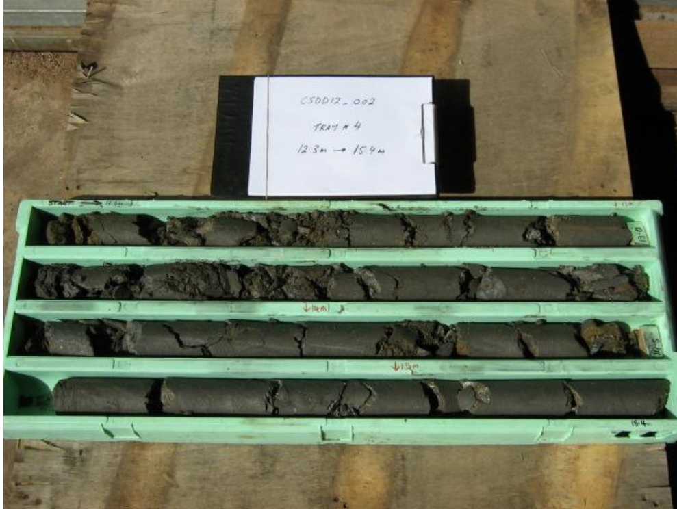
Plate 2. CSDD12_002 completely oxidised graphitic schist from 12.3 – 15.4m
