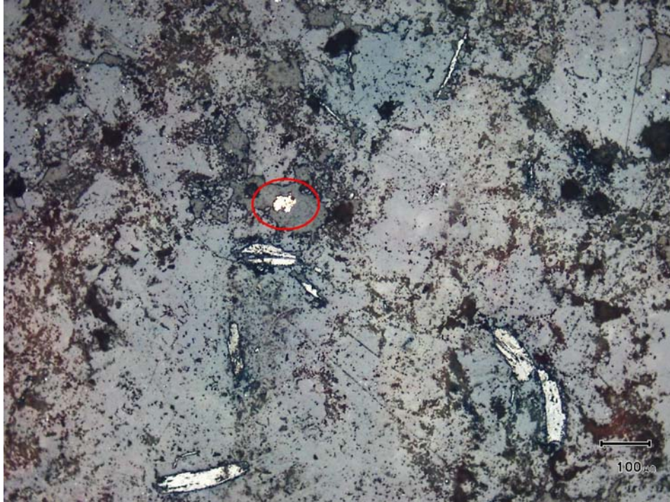
Figure 2. Carbonate breccia largely replaced by quartz, carrying a one grain of free gold associated with an equally fine soft grey metallic mineral which is possibly antimony.
