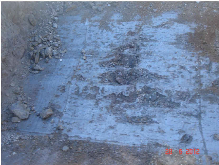
Plate 5. Close up of the drill sump for diamond drill hole CSDD12_003 showing massive intense graphite mineralisation.
