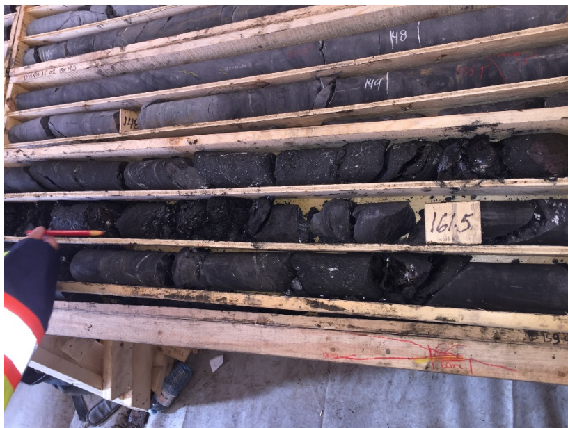
Panorama North core logging operation – coal intersection
