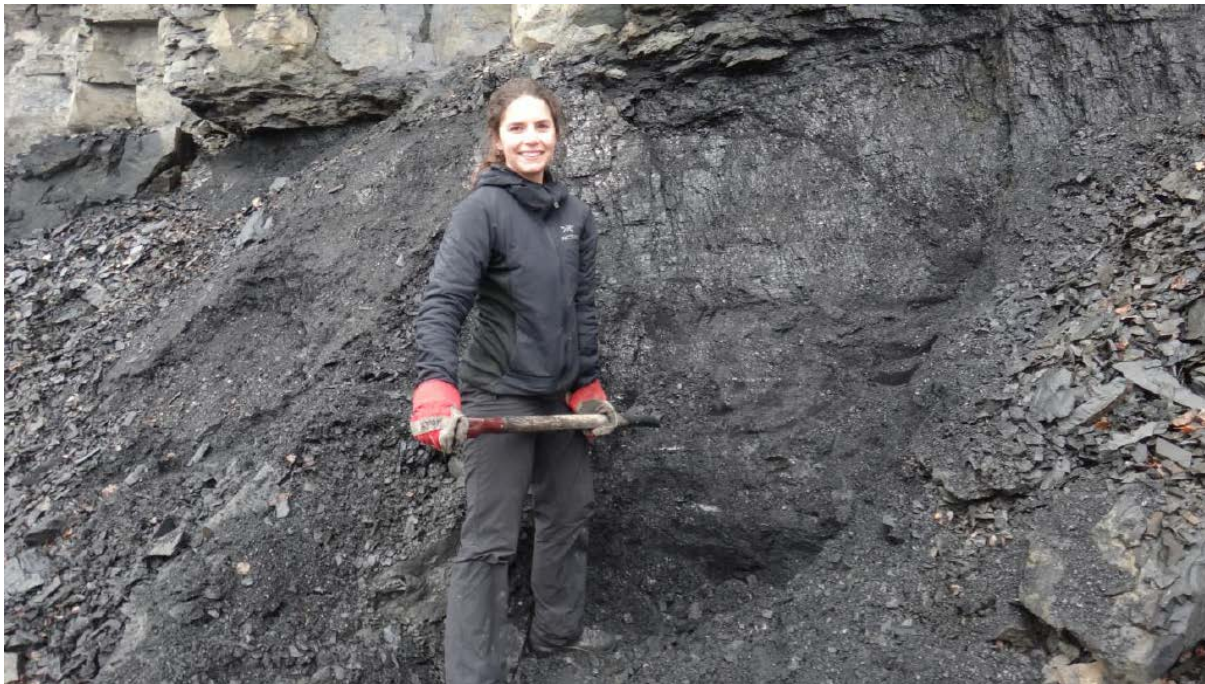
Plate 1. Channel sampling Duke E seam (insitu yields >80% at 10% ash)
