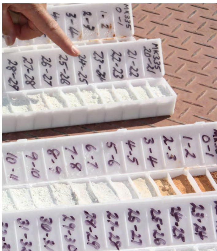
Drill holes up to 30m showing extensive kaolin
