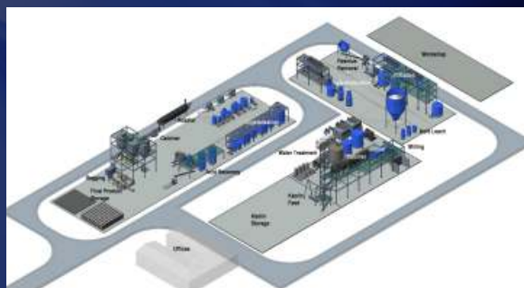
Figure 8 - HPA Plant General Layout and 3D View
