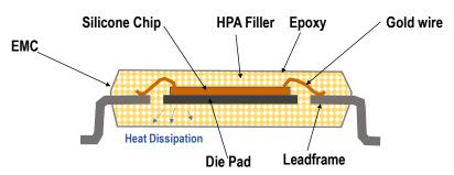
Figure 1: Schematic diagram of a SOP (Small Outline Package)
