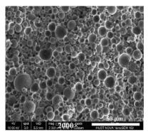
Figure 2 SEM Image of Alumina Filled EMC (50% v/v)
