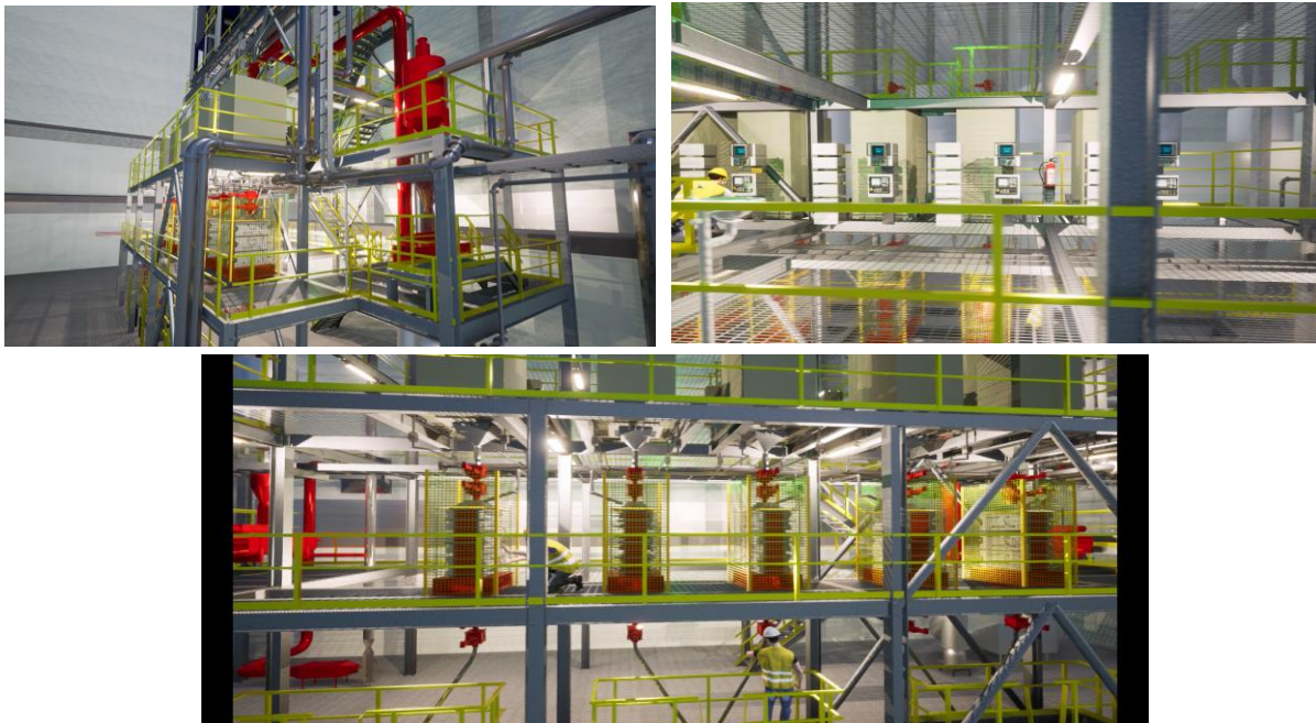
Figure 6 – In-house designed packed bed calciners
