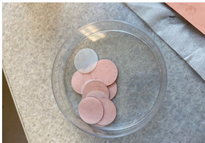
Figure 5: Preparation of anode component of the half-cell batteries
