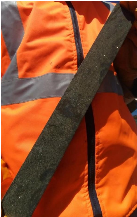
Figure 2. Section of diamond core from SWKRCDD034 (148m downhole) showing an interval of massive sulphide. The core diameter is 63.5mm.
