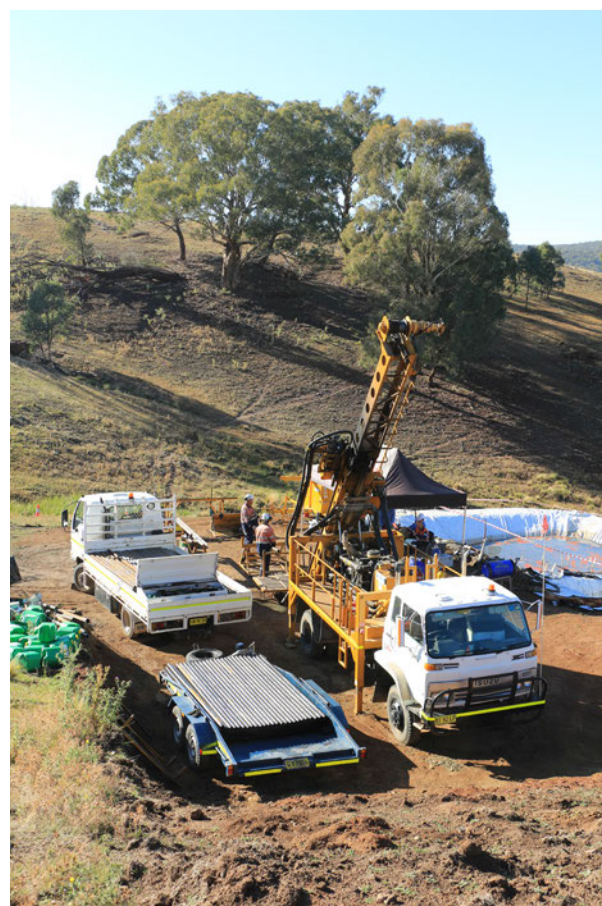
Figure 1 - Diamond drill rods in the process of being extracted from Hole # 2 and stacked on the trailer (foreground) in preparation for transport.
