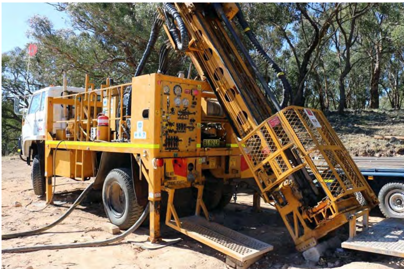
Figure 1 - The Warman 600 diamond rig at the Kempfield Hole #1 drill site
