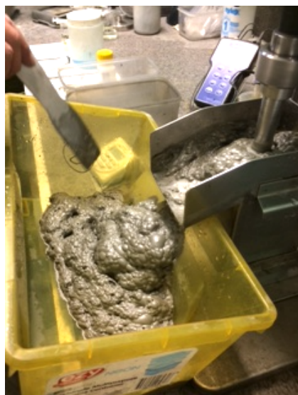
High grade (54-59%) zinc concentrate produced by the 2 nd cleaner stage of test AF8.
