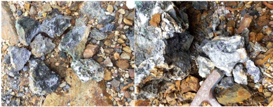
Figure 4 – Photos of rock chip samples ARDQ03 (LHS) and ARDQ04 (RHS) showing massive galena and minor chalcopyrite hosted by carbonate and shale
