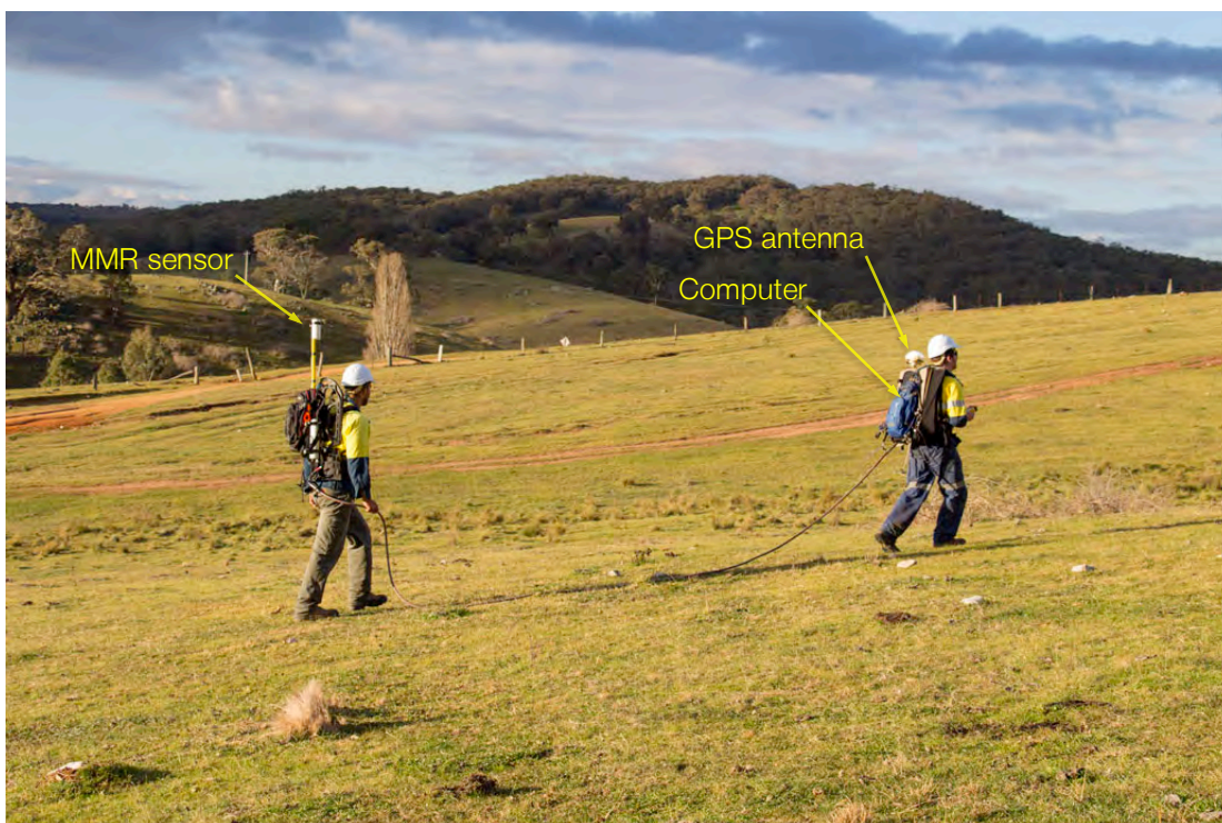
Figure 3 - Surface MMR survey in progress
