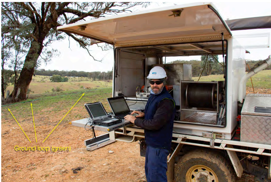
Figure 2 - MMR base station and ground loop
