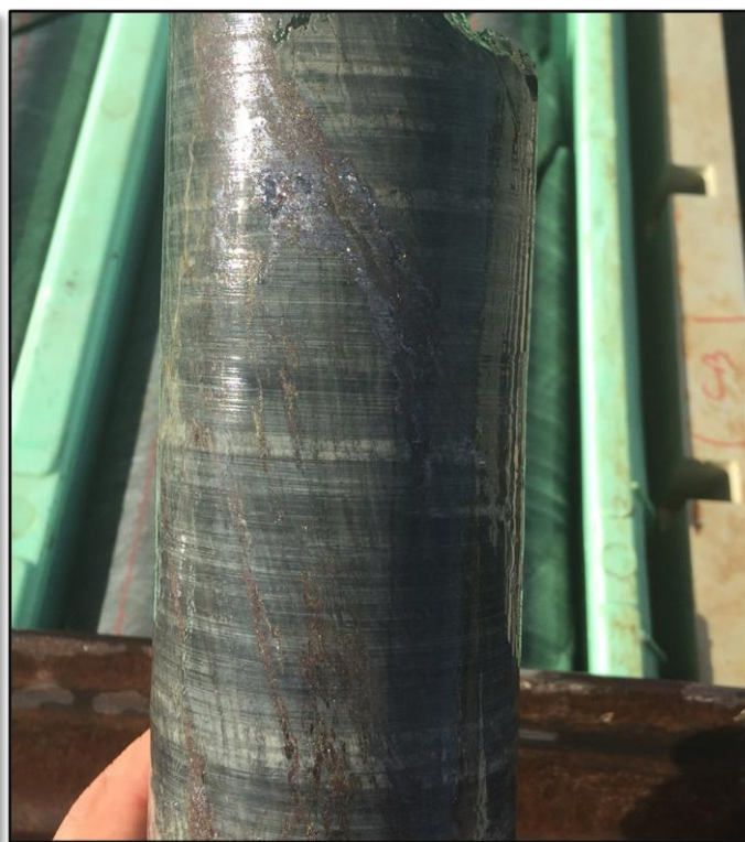
Drill core from HBRCD001 approx 490m, showing intense chlorite alteration (khaki colour) with zinc sulphide (brown) and lead sulphide (silver) mineralisation.
