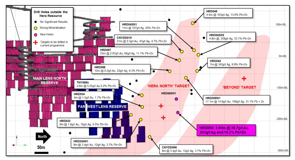
Long Section of the Hera North area (looking west) showing the new drilling results with respect to previous drilling and existing Reserves and existing Hera Mine development
