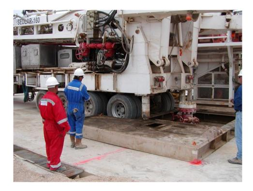
Sedlar - 160 drilling rig positioned above Sidi Dhaher #1 wellhead.
