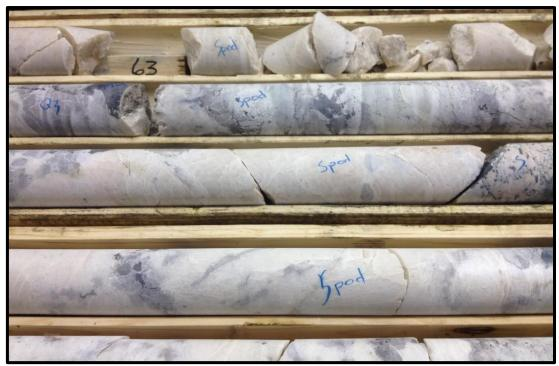
Figure 1. Drill core obtained from hole SL-16-73 showing a portion of the 15m intersection of high quality spodumene-bearing pegmatite.
