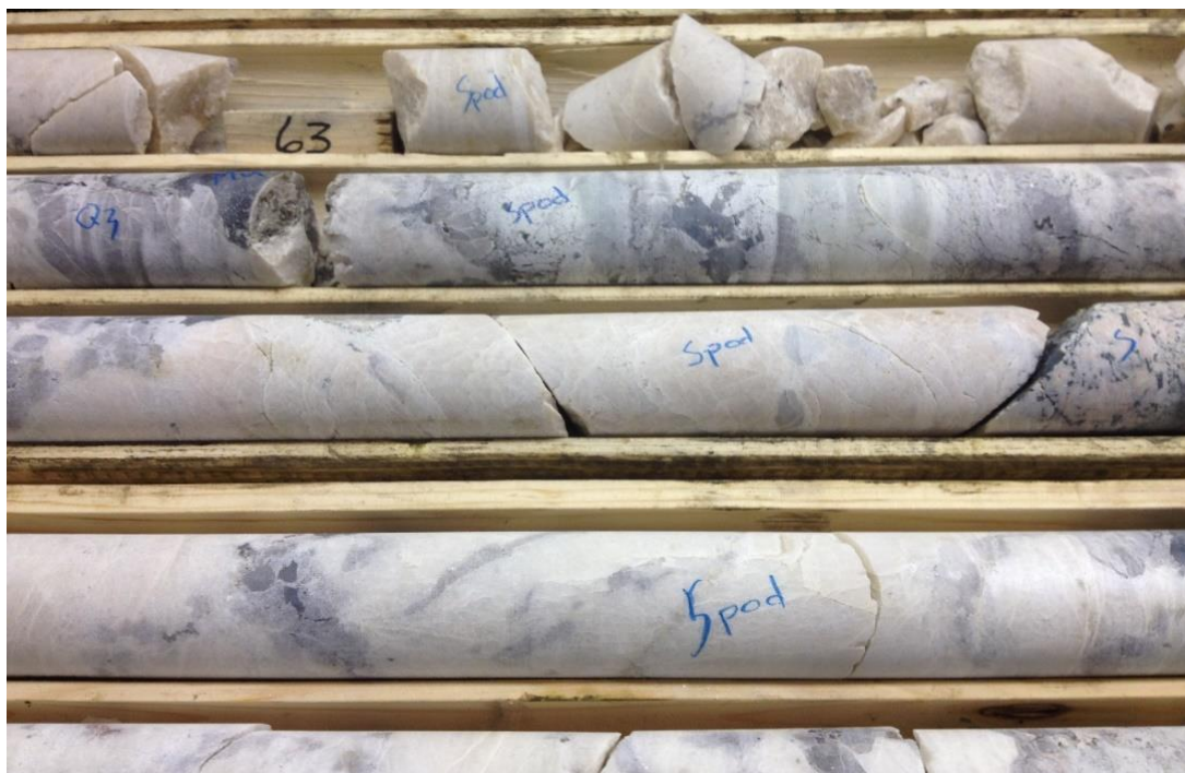
Figure 1. Drill core obtained from hole SL-16-73 showing a portion of the 15m intersection of high quality spodumene-bearing pegmatite.
