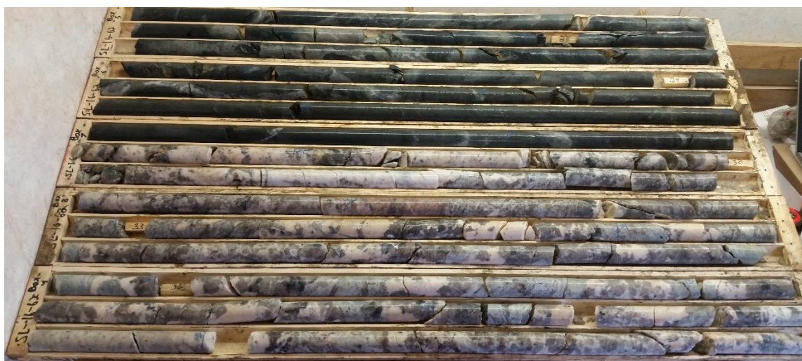
Figure 1. Drill core obtained from hole SL-16-62 showing an intersection of 12.06m of spodumene-bearing pegmatite.
