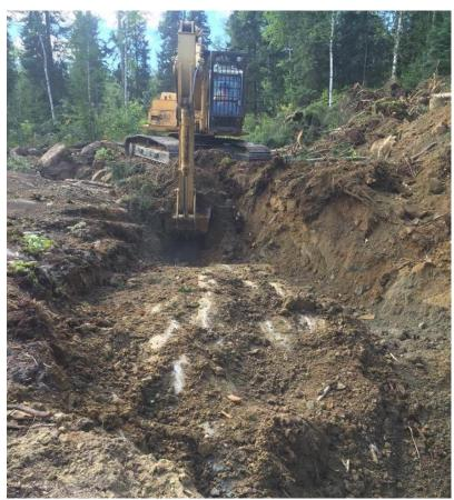
**Figure 3.** Excavator removing shallow alluvium cover from new pegmatite exposures located just south of the North Aubry prospect.
