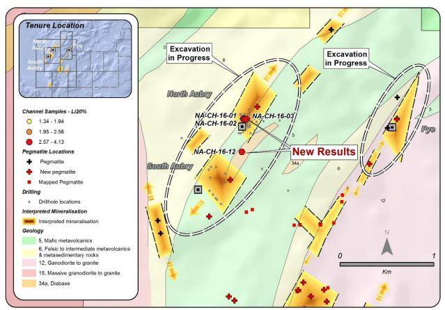
**Figure 2.** Overview of the Seymour Lake project showing the known and newly identified pegmatite exposures and the interpreted mineralised zones and structures. Also highlighted are some of the channel sample locations and the areas currently being excavated.
