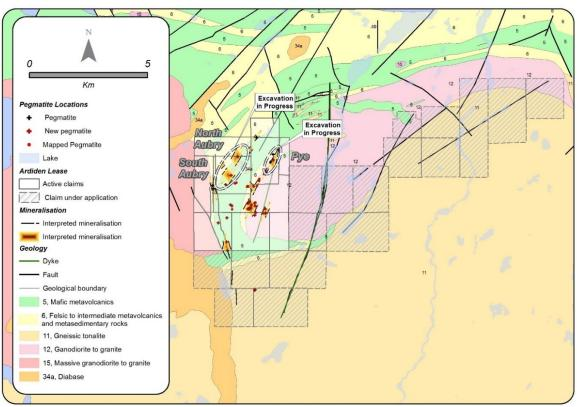
**Figure 8.** Seymour Lake Project overview showing new pegmatite exposures, faults and dykes and the newly staked claim areas.
