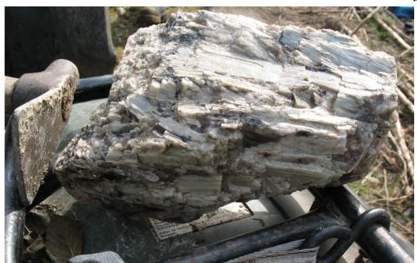
**Figure 5.** Example of high quality white spodumene crystals discovered during the excavations of pegmatite exposures south of North Aubry prospect.
