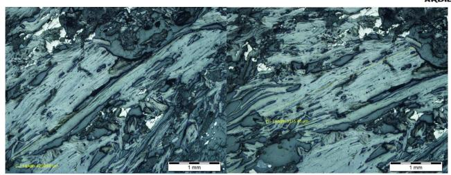
**Figure 15:** Petrographic slices from EM 12-05 – Flake size of 4,209 micron on left and 3,315 micron on right. Super jumbo graphite is defined as graphite with a flake size of >500 microns. (Source: Vancouver Petrographics, as announced to the ASX on 5 January 2016)
