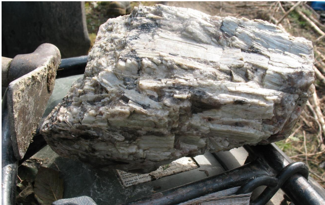
Figure 1. Example of high quality white spodumene crystals discovered during the excavations of pegmatite exposures south of the North Aubry prospect, Seymour Lake Lithium Project
