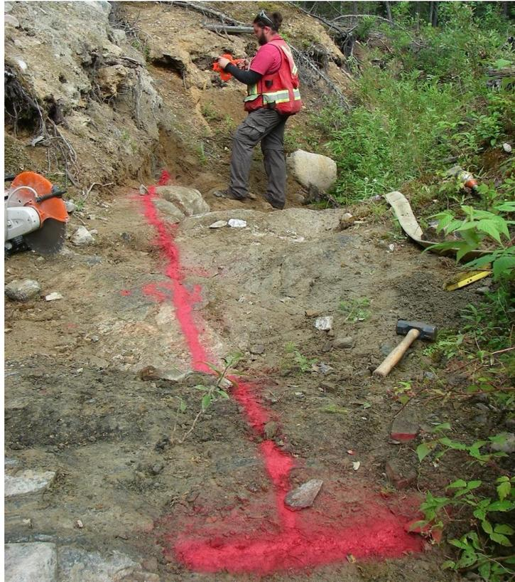
**Figure 6.** Excavation and preparation for channel sampling on the Root Lake pegmatite.
