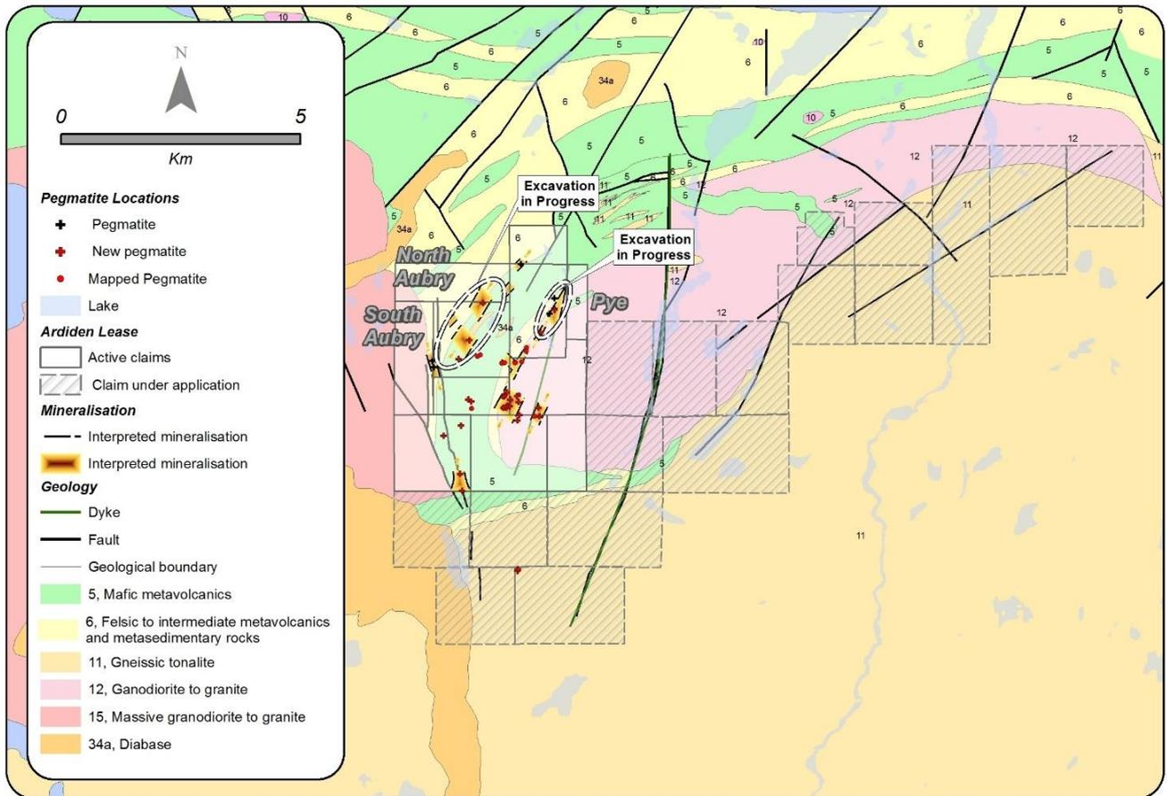
**Figure 1.** Seymour Lake project overview showing new pegmatite exposures, faults and dykes and the newly staked claim areas.
