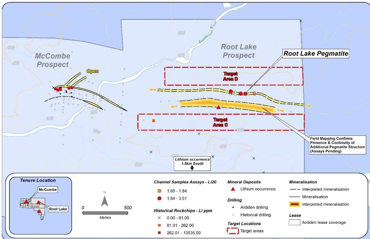
**Figure 9.** Overview of the Root Lake project showing the known and newly identified pegmatite exposures and the interpreted mineralised zones and structures. Also highlighted are some of the channel sample locations and the areas of interests for further exploration.
