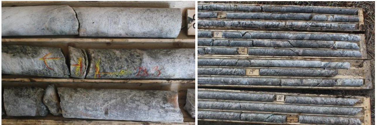
Figure 1. Drill Core from the Root Lake project showing multiple intersection of Spodumene mineralisation in the pegmatite structures.
