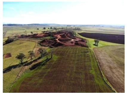
Figure 2: Rehabilitation at the Bald Hill Bauxite Project, Tasmania Rehabilitated land in the foreground and bottom right is now being cropped with good yields.
