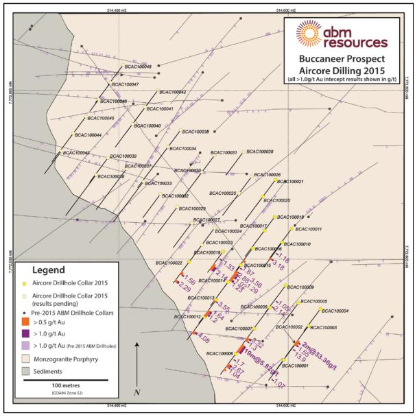
Figure 2. 2015 Buccaneer aircore drilling campaign plan view. Holes to the northwest are pending assays.
