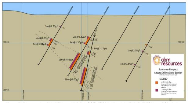
Figure 1. Cross-section SW-NE through hole BCAC100007. Note hole BCRC100058 was drilled at an acute angle to the cross-section and the separation between BCRC100058 and BCAC100007 is  $\sim$ 20m.
