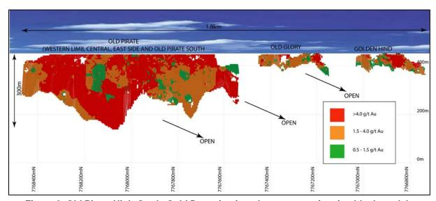
Figure 3. Old Pirate High-Grade Gold Deposit mineral resource estimation block model. Long section view ENE.
