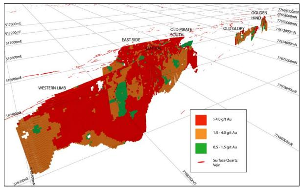
Figure 2. Old Pirate High-Grade Gold Deposit mineral resource estimation block model. 3D view SE.
