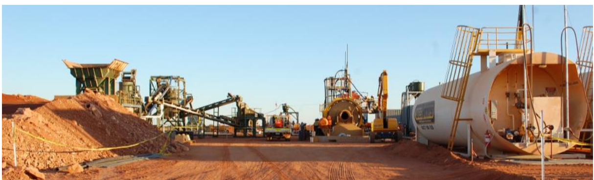
Figure 2. Wide-angle photograph of Pilot Processing Facility. Crushing circuit on the left, ball mill centre right (with Knelson concentrator behind) and fuel tanks / generators on the right.
